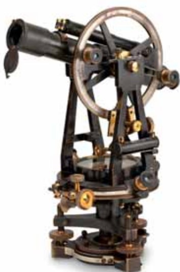
545 A 19TH CENTURY LACQUERED AND BLACKENED BRASS TRANSIT THEODOLITE ENGRAVED KELVIN & JAMES WHITE LTD, GLASGOW with two double silvered scale viewing lenses, 26cm wide, 20cm deep, 34cm high. £300 - 500 €390 - 650
